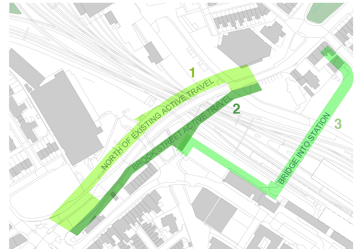
An additional walking and cycling bridge constructed in parallel to the existing bridge. Clearance enough to allow electrification of the railway lines beneath.
